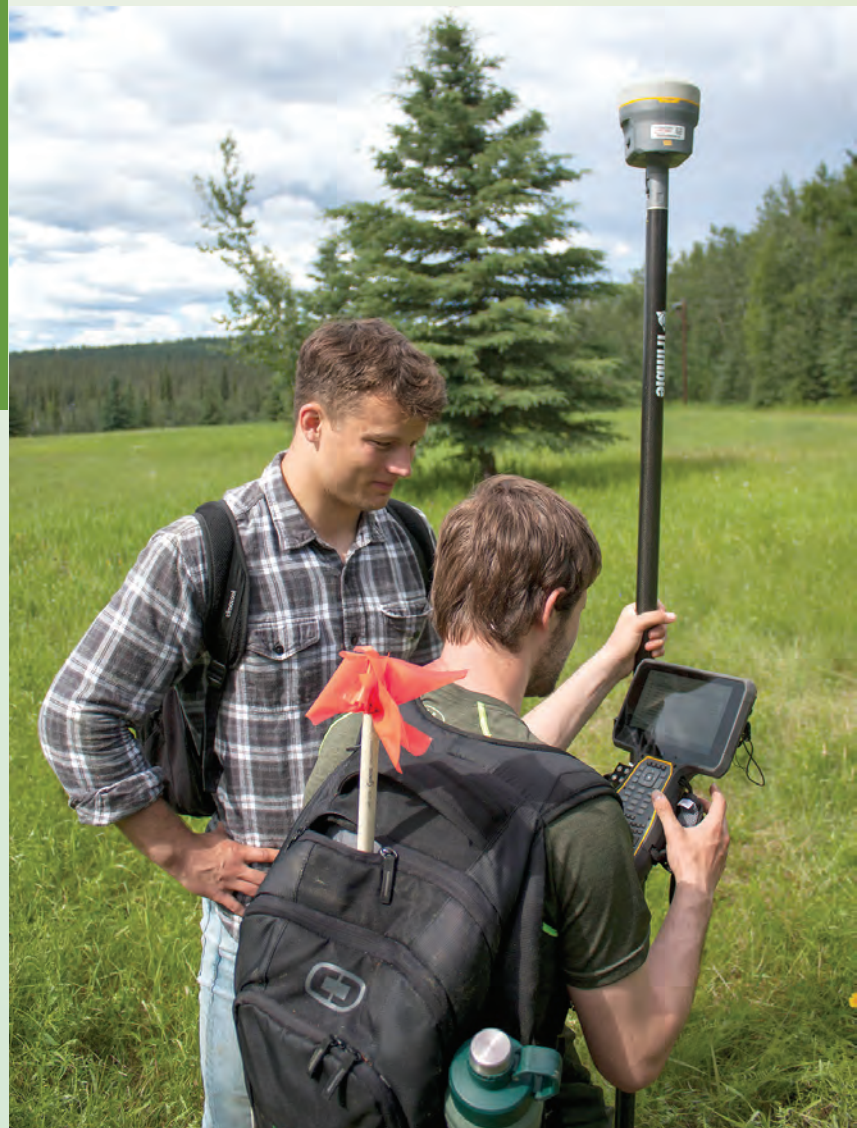
UAF graduate student Chris Smith, right, and UA Anchorage undergraduate Robert Haan check their GPS sensor while surveying 10-by-10-foot vegetation plots on the UAF North Campus trails. They're testing their field data against hyperspectral imagery of the same area as part of a project to improve remote sensing of fire fuels.
