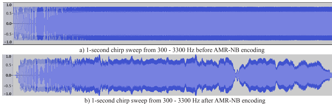
Figure 2: A comparison of a signal (a) before and (b) after being encoded with the AMR codec. Note that while the entirety of the signal is within the range of allowable frequencies for call audio, the received signal differs significantly from its original form. It is therefore critical that a high-fidelity mechanism for delivering data over a mobile audio channel be designed.
