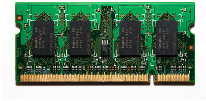
Figure 2: A SO-DIMM with its memory chips.
