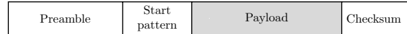
Figure 3: General packet structure of a rolling code. Gray background indicates that the part is either encrypted or authenticated.
