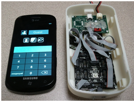
Figure 5: System prototype running on a WP Samsung Focus augmented with Gadgeteer sensors (white box).
