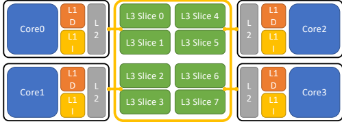
Figure 1: Diagram of Intel i7-7700 processor’s cache and core structure. Each core has its own L1 and L2 caches. The L3 cache is shared between cores, and is split into slices.
