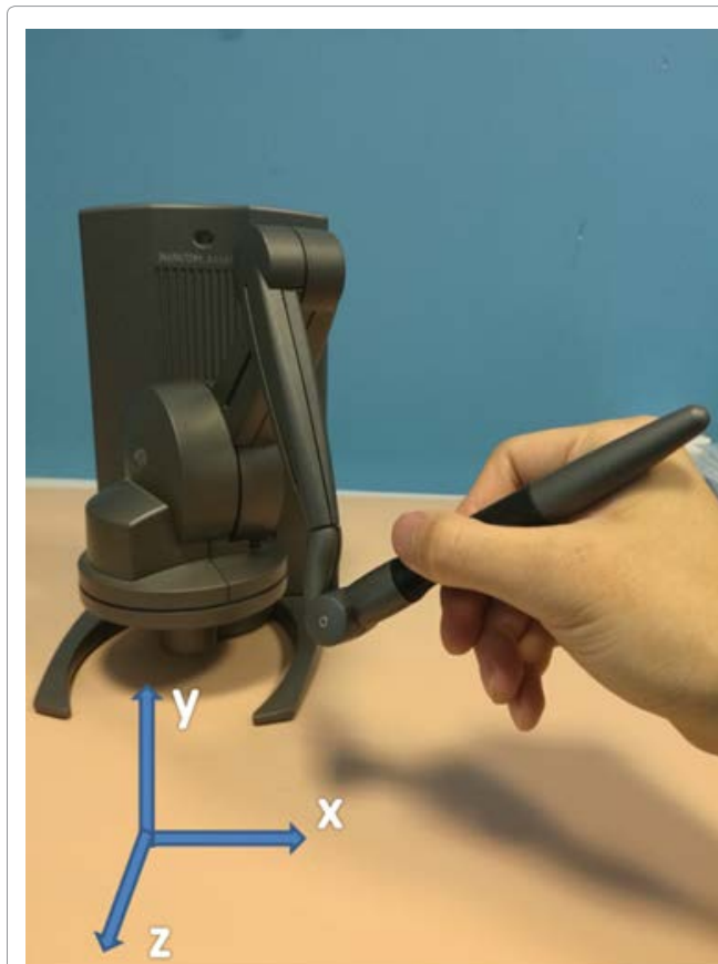
Figure 3: The haptic device used in this experiment, Geomagic Touch X and its workspace frame.
