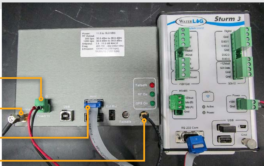
Figure 2: H-2221 Satellite Transmitter connected to a Storm 3 Data Logger
