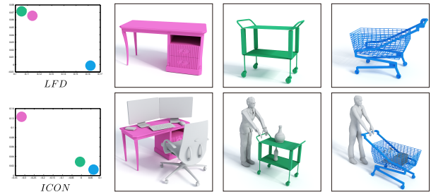
Figure 1: Similarity between shapes (top) vs. similarity between functionalities (bottom). A shape descriptor (LFD) considers the middle cart more similar to the desk, as shown on the left using a 2D MDS projection of the distances between objects. Our contextual descriptor, interaction context or ICON, takes into account object-to-object interactions and identifies the two carts as more similar.
