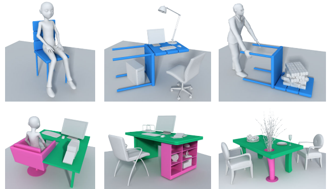
Figure 1: We learn how a category of 3D objects function. This may lead us to discover that the geometry of a chair could allow it to function as a desk or handcart (top). One could produce functional hybrids (bottom), where different functionalities discovered from two objects are integrated into a multi-functional product.
