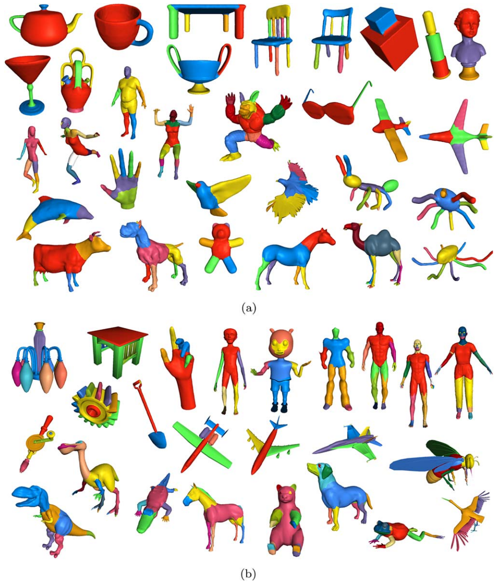
Fig. 9 Partitioning to parts using the SDF results works on a wide variety of models, as seen here for sample models from the SHREC model set (a), the PSB, and other sources (b). All the results seen above were achieved automatically with a small (4) number of Gaussians fitted to SDF histograms
