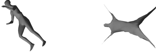
Figure 2. A human mesh (left) and its 3D spectral embedding, constructed using the second, third, and fourth eigenvectors. This particular choice of the eigenvectors is explained in Section 5.
