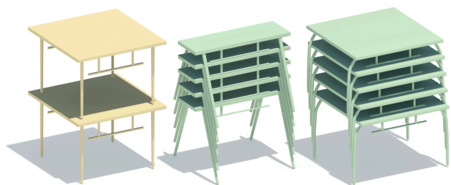
Figure 11: Two different stackabilization solutions for the table are obtained by using cuboids or GCs to fit the legs respectively. These two solutions have the same stackability ( S = 0.8 ), but introduce rather different distortions to the shape geometry and functionality.
