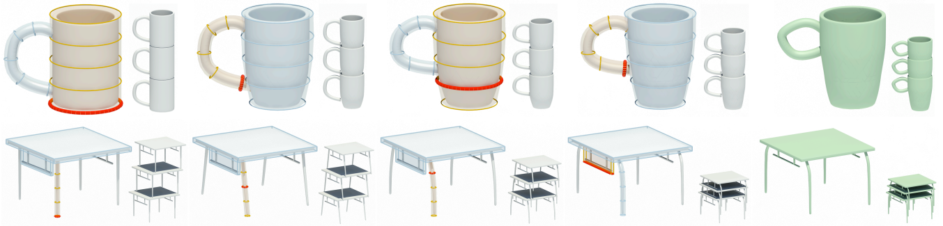
Figure 8: Progress of stackabilization on a mug and a table model. During each iteration, contact parts (in orange) and active deformation handles (in red) are detected. Contact-driven deformation is applied to the shape to improve its stackability.
