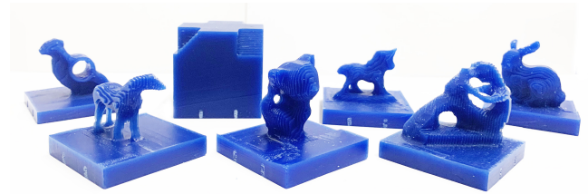
Fig. 27. Rough CNC machining results of some of the models shown in the paper. The CNC machine was set to carve the carvable volumes produced by our decomposition algorithm, following the carving directions computed. Each volume is carved using a connected Fermat spiral toolpath.
