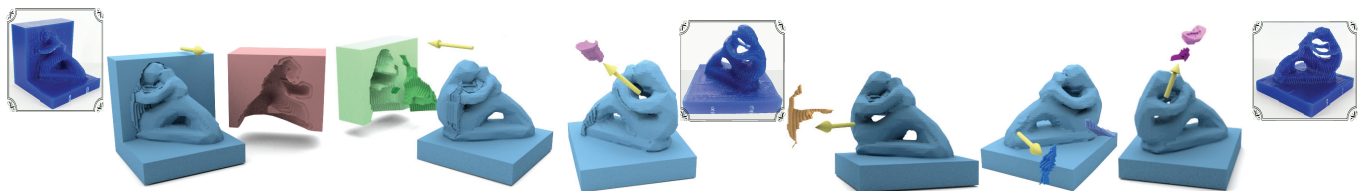
Fig. 1. Carvable volume decomposition computed by our algorithm for the high-genus Fertility model, with 6 carving directions (indicated by the yellow arrows) and a total of 10 carvable volumes (one carving direction may yield multiple volumes, e.g., 3 volumes for the second direction). Three insets show physical outputs produced by CNC rough machining. Each carvable volume is continuously carved following a connected Fermat spiral toolpath.
