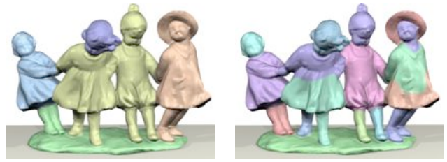
Figure 3: Results of a conventional mesh segmentation scheme [Liu and Zhang 2007] based on the minima rule (use of concavity) are not so meaningful. Left: 5 parts (compare with Figure 1(d) for an IRSA-induced segmentation also having 5 parts). Right: 16 parts.
