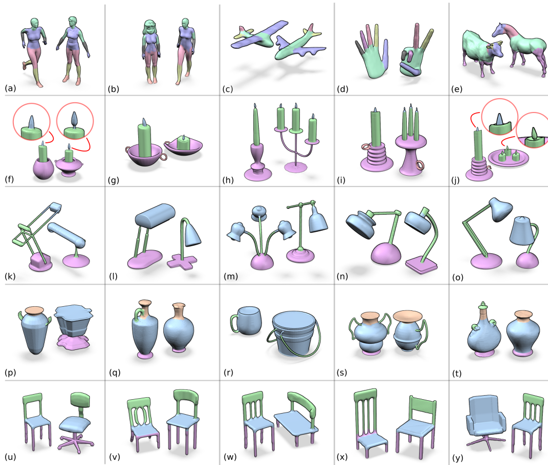
Figure 5: Part correspondence results via joint labeling. Aside from the failure cases in (j), (t), and (y), our method succeeded even under significant geometric and topological variations between the matched parts, while purely content-driven methods would fail (see Figure 7 for a comparison). Corresponding segments between a pair of shapes with the same color.
