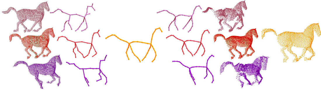
Figure 1: Overview of our consensus skeletonization workflow. Left to right: From an initial set of deforming point clouds, we extract skeletons per frame. We compute the consensus skeleton (middle) and deform it back to the frames' poses. Using the skeleton correspondence, we can deform the point clouds into a common consensus pose and register them together (right).
