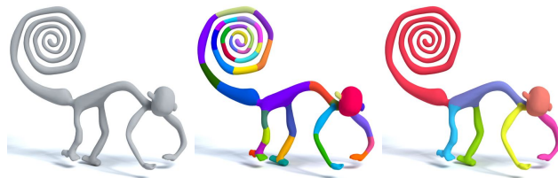
Figure 1: Generalized cylinder decomposition obtained by our algorithm (right) produces considerably fewer parts compared to approximate convex decomposition (middle).
