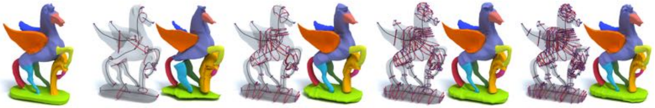
Figure 22: Progressive shape approximation using generalized cylinders from our decomposition algorithm. The pegasus model from [Thiery et al. 2013] is decomposed (leftmost) into 11 parts. A set shape approximations are generated (from left to right) through progressively increasing the number of profile curves and control points ( \#P , \#C ) from (25, 100), (50, 300), (75, 600), to (100, 1000). The approximation errors ( H , M12 , M21 ), as defined in Table 2, decreases from (6.188, 0.813, 0.683), (2.139, 0.311, 0.32), (1.456, 0.192, 0.198), to (1.456, 0.151, 0.156).
