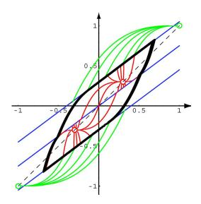
Fig. 3. Two-bit (four-level) quantized implementation of constant gain feedback control in the case  $|k_1|/k_2 < 1$ . Specifically,  $k_1 = -2$ ,  $k_2=8/3, r=0.3$ , and s=0.8. Design is not regular and this results in existence of limit cycle (black curve) which is both large, relative to the operating region, and persistent, as length of sampling interval h tends to zero.
