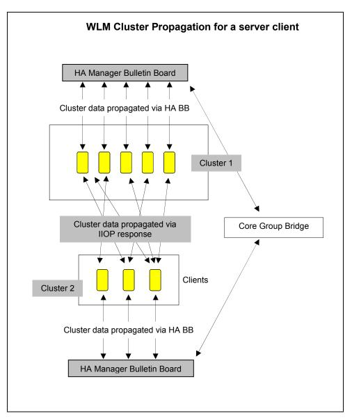
Figure 4: WLM cluster propagation for a server
