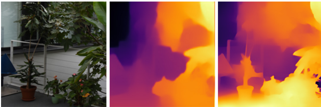
Figure 4: We complement the upsampling results from MiDaS [5] from Figure 5 of main paper here with matching results from SGR [7]. The original image with resolution 192 \times 192 gains additional details in the depth estimate when fed to the network after upsampling to the receptive field size of 448 \times 448 (right) instead of its original resolution (middle).
