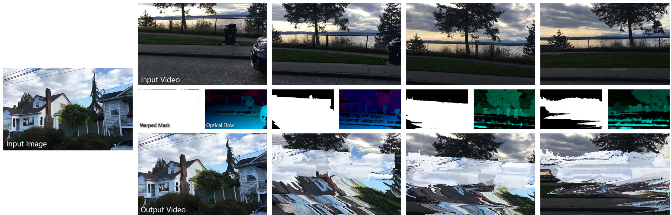
Figure 2: Our algorithm in its simplest form operates on an image and a video sequence. We compute the optical flow of the video sequence and use the motion to warp the pixels of the input image. We keep track of any holes created from warping using a binary mask, the warped image is composited with each from of the input video to create a data moshed output video.
