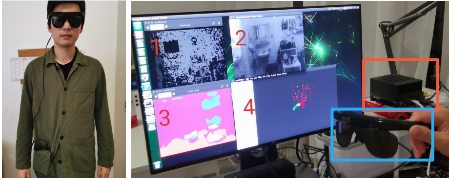
Fig. 2. Devices and the real-time results of our system. The left image shows the user wearing the devices. The blue box in left image indicates the smart glasses while the orange box indicates the Xavier processor. The windows on the screen exhibit (1) the depth image, (2) the input frame for the SLAM system, (3) the semantic segmentation result and (4) the 3D map.
