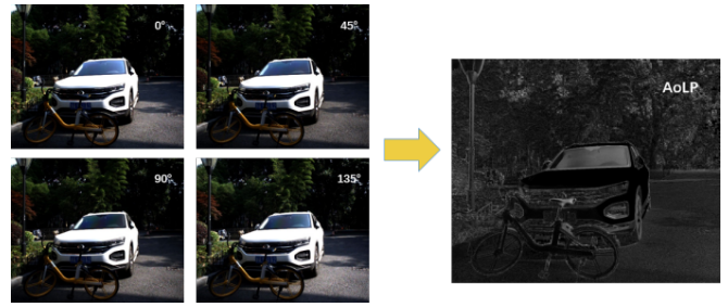
Fig. 7. Preprocessing of Polarization image: (a) RGB images at four directions and (b) Polarization image.
