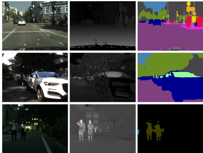
Fig. 1. Examples of images and recognition results: (a) RGB image, (b) Multimodal image (From top to bottom: depth image from Cityscapes [7], polarization image from ZJU-RGB-P [8], and thermal image from MFNet [9]), (c) Segmentation result using only RGB image.
