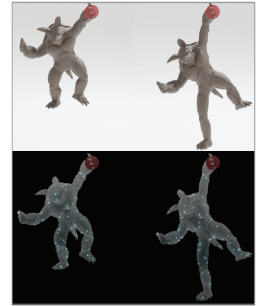
Fig. 11. We drag the left leg of the Armadillo. Neural Cubature with 140 elements runs the simulation robustly. We also visualize the weight value at each Cubature element. Higher weighted elements are brighter. Greedy Cubature fails in this simulation.
