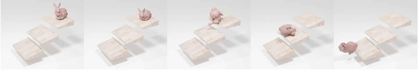
Fig. 13. Falling bunny. We use generalized Newton-Euler equation to couple DAE-based model reduction with large rigid body motion to simulate free-floating objects. The subspace configuration of the bunny is n_p = 30 and n_q = 10 .
