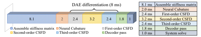
Fig. 12. Detailed time breakdown of our DAE-in-the-loop simulation pipeline. The timing information is for the dinosaur model with a 9-layer decoder net.
