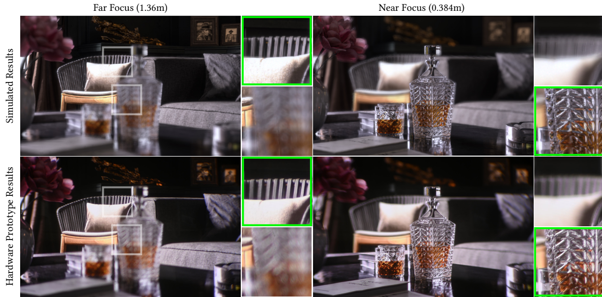
Fig. S6. Simulated vs experimental results on our Split-Lohmann lab prototype. (Credits: 3D scene courtesy of “Entity Designer” at Blender Market)
