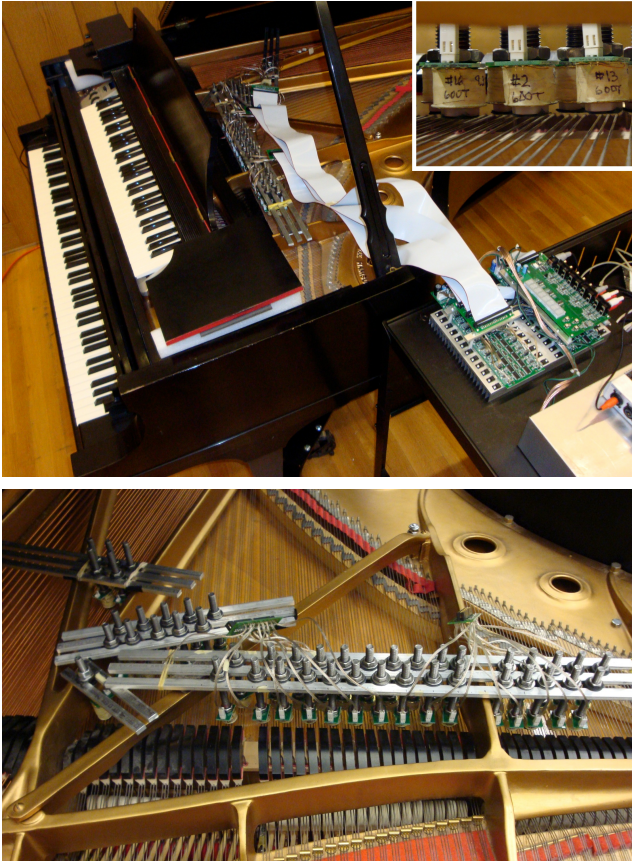
Figure 1: The magnetic resonator piano. Top: complete system. Top inset: electromagnetic actuators above the strings. Bottom: Brackets holding actuators for four octaves of strings.
