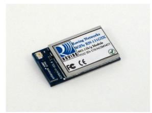
Figure 5. The WiFly 802.11b/g radio module.
