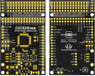
Figure 2. Top and bottom renderings of the latest CUI32Stem – it is very similar to the current CUI32, but swaps the generic prototyping area in favor of 4-pin connectors for SeeedStudio's GROVE system, allowing sensors and actuators to be attached - no need for solder
