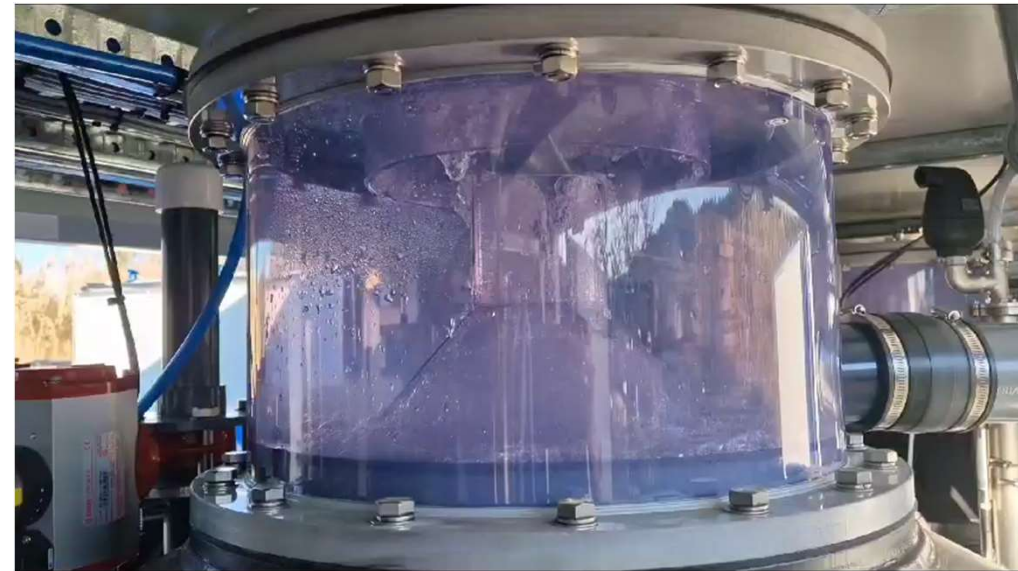
Primary Fractionation of raw groundwater
