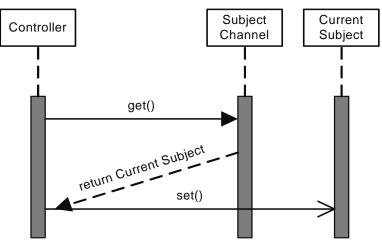
Fig. 3: The Proxy Pattern in extended MVC Architectures with Subject Channels
