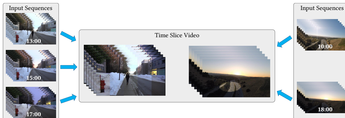
Fig. 1. Time slice video makes use of a robust spatio-temporal alignment to enable the blending of multiple videos recorded with different appearances to be blended together in a number of configurations. Here we show traditional time slice vertical bars (left), as well as a world-space shape that drives the compositing, such as the 3D spotlight (right).
