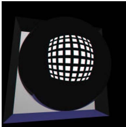
Figure 2.8: Raytraced sphere One of the 40 computer generated images used for the reconstruction of a specular sphere.
