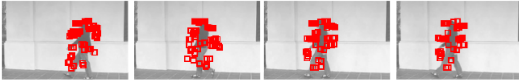
Figure 2.8: Illustration of interest points of a walking action by Dollar's detector [Dollar et al., 2005]. This figure is reproduced from [Niebles et al., 2008]
