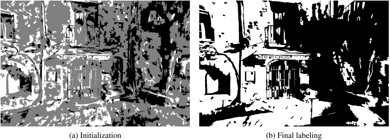
Figure 3.4: (a) Initial labels from unary term, white is in light, black in shadow and grey undefined. (b) Final labels after convergence.
