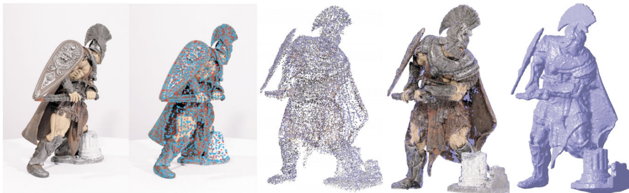
Figure 2.3: Overall approach from [Furukawa and Ponce, 2007]. From left to right: a sample input image; detected features; reconstructed patches after the initial matching; final patches after expansion and filtering; polygonal surface extracted from reconstructed patches.
