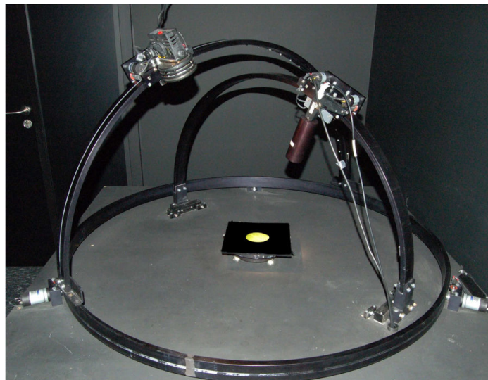
Figure 2.28: A gonioreflectometer measuring the BRDF of a planar sample by sampling the double hemisphere of incoming/outgoing radiance using a directional light source. [Li et al. , 2005]
