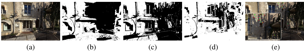
Figure 3.3: The consecutive steps of the algorithm to determine L_{\text{sun}} for the “Street” scene. (a) Input image (b) shadow from inaccurate 3D model: the proxy overestimates the geometry of the cactus and creates a “blob” shadow (c) K-means intensity estimation: some black areas are not shadows (d) intersection of (b) and (c): a more reliable subset of shadows are found, which are used in (e) to find pairs used to calibrate the sun.
