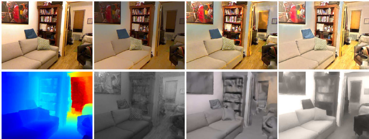
Figure 2.15: Intrinsic decomposition of an RGB-D image from the NYU Depth dataset [29]. First column Input color and depth image. Albedo and shading images estimated by two recent approaches for intrinsic decomposition of RGB-D images [Lee et al. , 2012], [Barron and Malik, 2013a] and by [Chen and Koltun, 2013].
