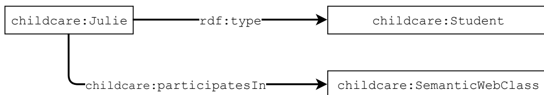
FIGURE 1.1: RDF graph that describes the sentence Julie is a student and Julie participates in the semantic web class along with the used prefixes
